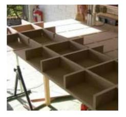
Apart from cutting the cross-halving joints as accurately as possible (so that there was no "slop" in the resulting joints), the use of the shallow dados really helped to register the core with both the top and bottom of the box, preventing any racking or sliding when assembling. It really was well worth the effort!
