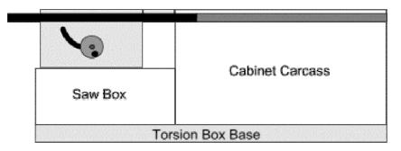
Here's a simplified front view of one possible cabinet format. The standard rails are shown black, with the additional (full-length) rails shown gray. The major consideration here is the overall width and this is affected by other considerations, which must be made at an early stage, such as:
