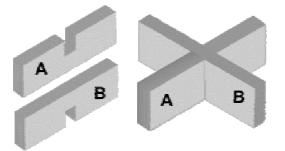
Rib "A" is notched halfway through, as is Rib "B" - the width of the notch equal to the thickness of the material. They can then interlock, as shown, when "B" is lowered over "A" at right angles.
