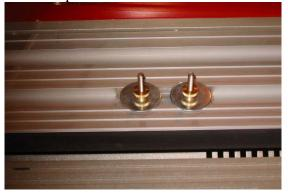
7. Now we just need to attach whatever we want to the holder put it in the slot and tighten it down. As you can see from the pictures below I am using this one to hold one of my poly featherboards.
