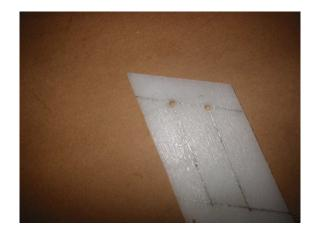
5. Next using a straight bit in your router cut your mounting slots. Be careful of the router speed as the router can melt the poly. Then clean up the mounting slots. You are finished with the board and it will look something like this:
