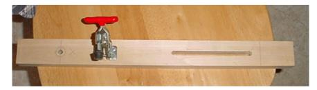
Cut a piece of 1/2" plywood 10" by 18". With a router mill a slot 5/16" by 8" 4-1/2" from one edge leaving 1" on each edge. Centered on this slot mill another slot 1/2"wide 1/4" deep. This slot will hold the lower fence mounting bolt's head. This part will be your backer board. While making these cuts you will also want to cut a piece of 4/4 hardwood 4" by 2" to attach the threaded rod to the backer board later.
