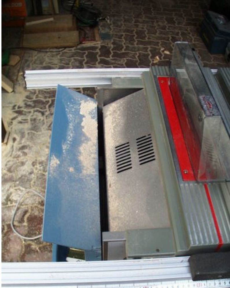
Sawdust Goes Down Between Box and Body, Into Pan
