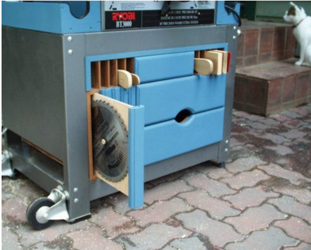
Saw Blade Racks Slide in Grooves
