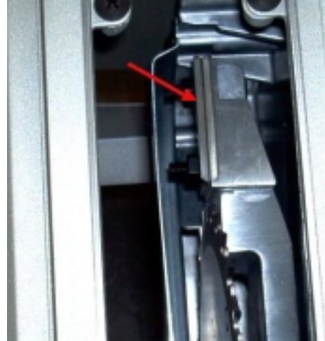
The improved BT3100 splitter shims
