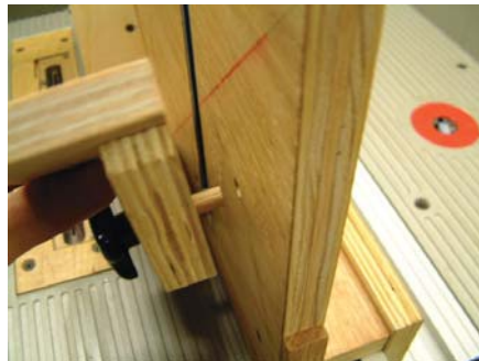
Insert the dowel into the predrill hole
