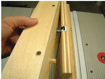
Install the fences on the T-Track
