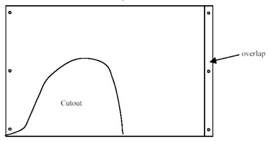
Sheet 10. high by 15-17/32 wide. This allows  $\frac{1}{2}$  for overlap; the circumference of the inlet is 15-1/32.
