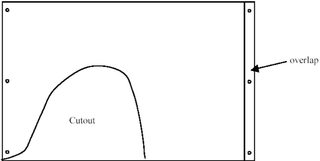
Sheet 10. high by  $15-17/32$  wide. This allows  $1/2$ . for overlap; the circumference of the inlet is  $15-1/32$ .
