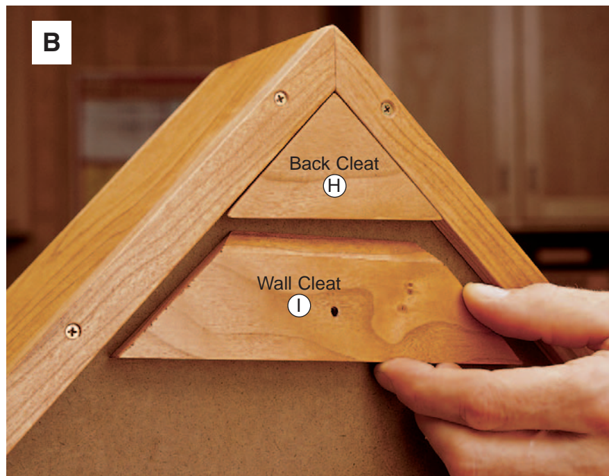
The mating cleat bevels provide concealed attachment. Level the wall cleat during installation to ensure a level-hanging case.
