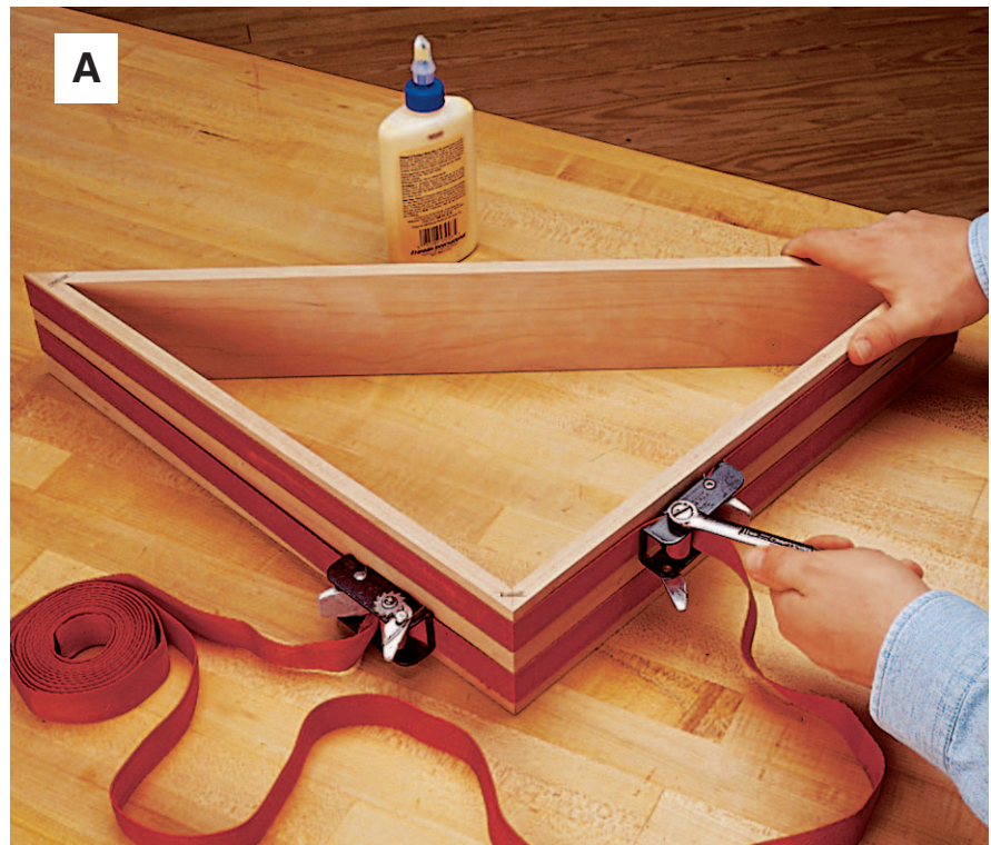
Set the assembled frame on a flat surface, and draw its mitered corners together with a pair of bandclamps.
