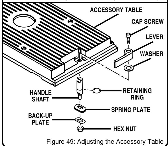
Figure 49: Adjusting the Accessory Table
