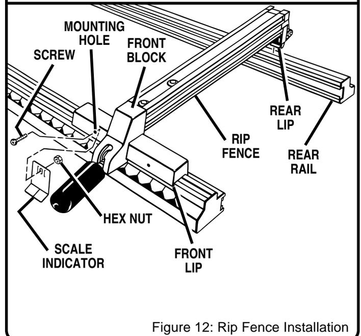
Figure 12: Rip Fence Installation
