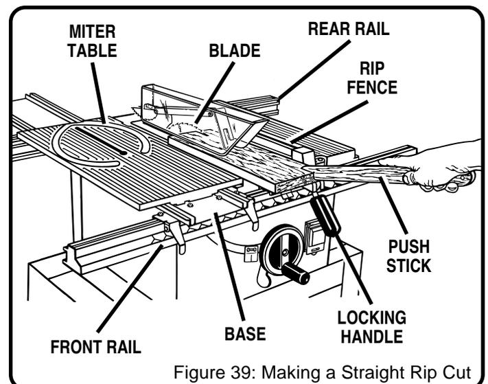
Figure 39: Making a Straight Rip Cut
