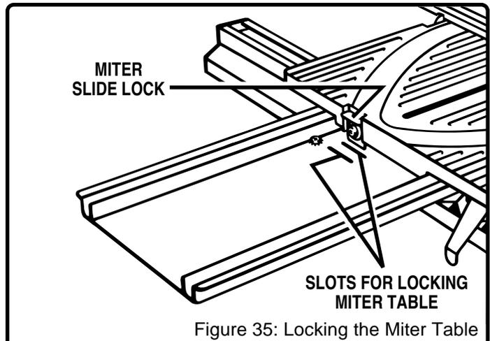
Figure 35: Locking the Miter Table
