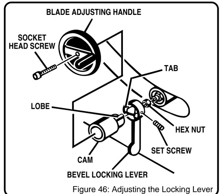
Figure 46: Adjusting the Locking Lever
