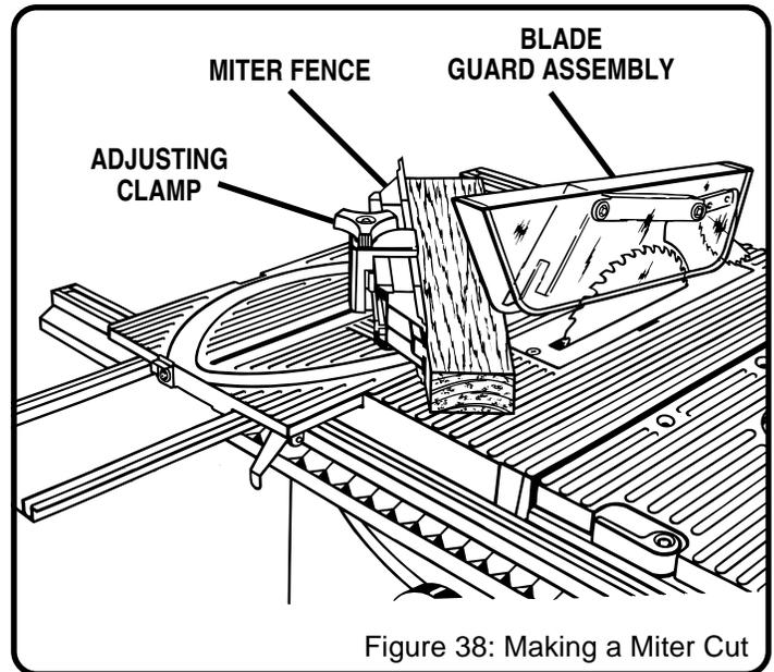
Figure 38: Making a Miter Cut
