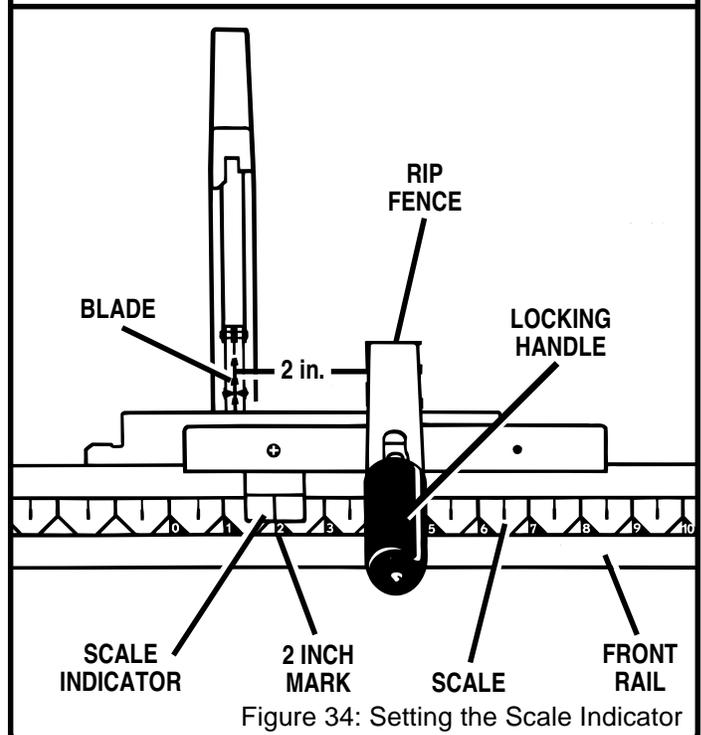
Figure 34: Setting the Scale Indicator
