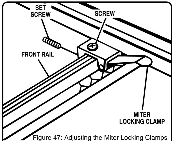
Figure 47: Adjusting the Miter Locking Clamps
