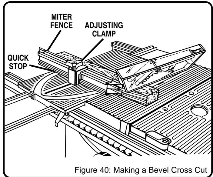
Figure 40: Making a Bevel Cross Cut
