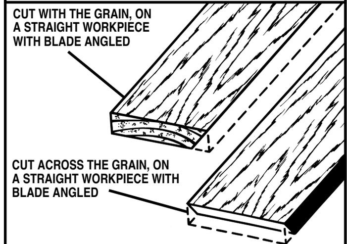
Figure 21: Bevel Rip Cut And Bevel Cross Cut
