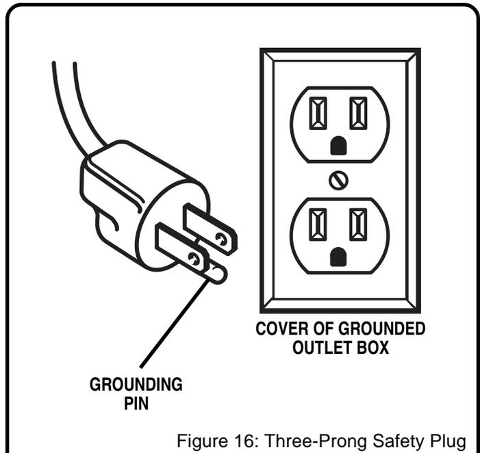
Figure 16: Three-Prong Safety Plug
