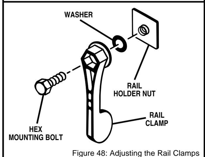
Figure 48: Adjusting the Rail Clamps
