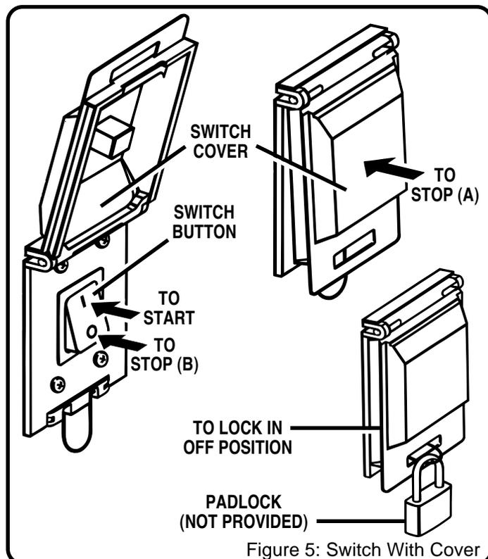
Figure 5: Switch With Cover
